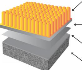
Carbon negative Thrive® Matter Nylon 6 fibre. Made with 100% post-industrial recycled resin. Constructed for optimum wear performance and appearance retention.
